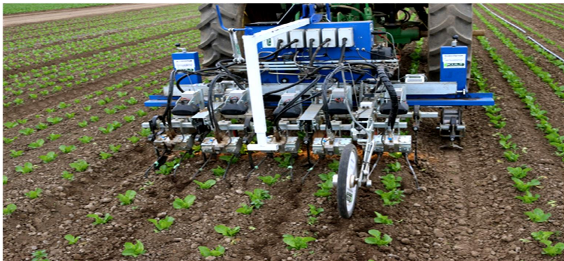
Figure 2. Robovator automatic intra-row cultivator in a commercial lettuce field near Santa Maria, CA. The reciprocating cultivator knives, shown open, move in an out of the row removing weeds between the crop plants. Photograph by Steve Fennimore.
