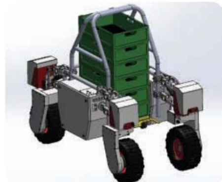
FIGURE 3 The initial trial of a robotic strawberry transportation system in polytunnels (left) and a dedicated design for an on-board picking tray storage (right).
